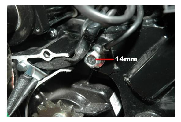
On the left side of the engine use a 14mm box wrench to hold the engine mount bolt.
