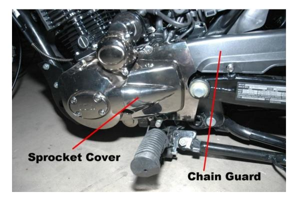
Remove the chain guard bolts (10mm) and slide the guard towards the rear of the bike a few inches. Remove the sprocket cover bolts (8mm) and remove the cover. It is not necessary to remove the shift lever.
