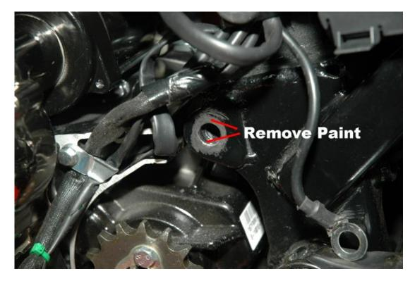
Using a small die grinder or a Dremel with a wire brush attachment, remove the paint around the bolt hole.
