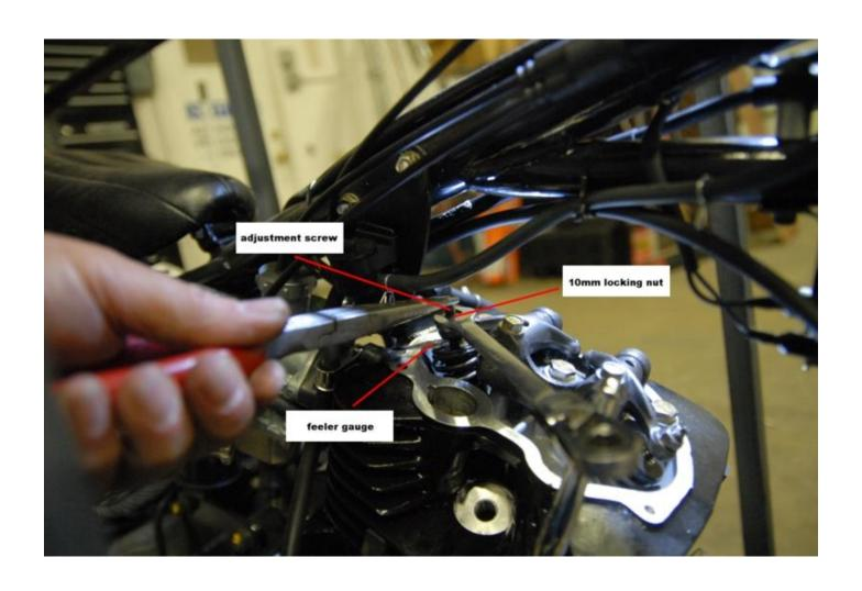
Image showing the feeler gauge inserted between the base of the adjustment screw and the top of the valve stem for clarification. Note it is easier to use the gauge if you remove it from it's holder. Feeler gauge sets are available form most auto parts stores.
