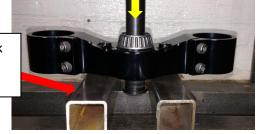
3. Remove the lower steering bearing, washer, seal and steering stem.
