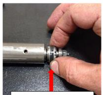
Compress the piston seal when installing
