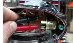
If the brake light illuminates from **only one brake** (either front brake or rear brake), disconnect the brake switch at its connector and jumper a wire between the connector terminals. If the brake light illuminates, replace the faulty switch.
