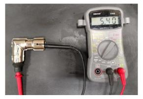
Disconnect the BLACK/YELLOW wire and measure the resistance of the primary (low voltage) side of the coil with an Ohms meter. Typical resistance 0.4 Ohms.
