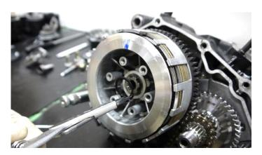
Lift off the clutch center, pressure plate and clutch plates. Lift off the thrust washer and clutch basket.
