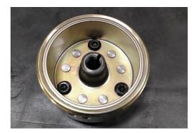
The starter clutch, cams and gear with hub should be replaced as an assembly. Insert the cams and friction ring into the clutch outer as shown. Note that the ring flange and flange split will face the flywheel. Install the clutch onto the flywheel with the 3 x M8 bolts. Apply medium strength thread lock and tighten the bolts to 23N-m.
