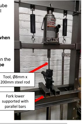
6. The lower tube cap may be removed with an impact gun. The cartridge is attached to the lower fork cap and the cartridge will be removed with the lower fork cap. Extract the cartridge from the lower fork tube.
