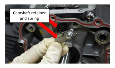
2. Extract the camshaft **spindle** and **thrust washer** from the left. Lift out the **camshaft**. Inspect the camshaft bushing for galling or excessive wear. Inspect the cam lobe for galling or excessive wear. Replace if damaged.
