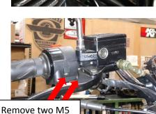
Remove two M5 screws on switch
