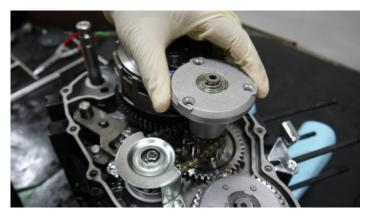
5. Be sure that the gasket sealing surfaces are clean and flat. Install the right side engine cover with a new gasket. Hold the clutch lifter arm in the position shown (against the spring pressure) during installation. Verify that the 2 x 10mm locating dowel pins are present in the crankcase. Fasten with the 13 x M6 bolts. Tighten the bolts progressively to 11N-m. The clutch cable bracket is installed in the location shown.
