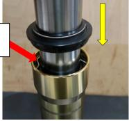
**12.** Fill the fork with **270cc** of **10W fork oil**. Pour slowly and stroke the cartridge rod to bleed out air from the cartridge.
