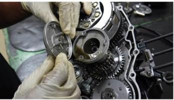
4. Remove the oil filter nut and concave washer with a 24mm ID lock nut tool. Remove the filter housing.
