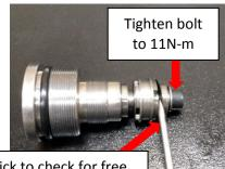
Use a pick to check for free movement of the check shim
