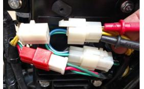
For an open circuit or short to ground, remove the engine sprocket cover and inspect for damaged wires.
