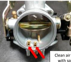
**1.** Clean the exterior and interior of the carb body with cleaner and a soft brush.
