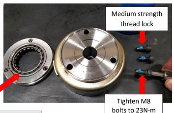
Alternator and Left Engine Cover Installation
