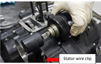
Remove the 8 x M6 bolts fastening the left side engine cover. Remove the cover with stator. Remove the neutral switch, fastened by 2 x M6 bolts.
