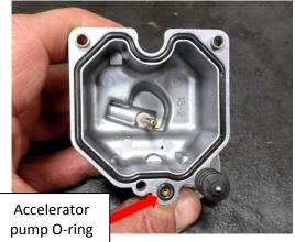
7. Install the **float bowl**. Be sure that the accelerator pump **cam arm** is in the UP position. Install the three float bowl **screws**.
