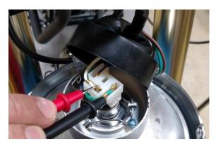
If battery voltage is low or not present in either Hi or Low circuits inspect the left handlebar Hi/Low switch for damage or corrosion.
