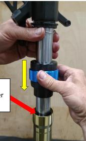
**13.** Install the **fork spring, spring guide** and **washer**. Hold down the spring guide to install the cartridge rod **M10 nut**. Screw the nut down to the bottom of the threads.
