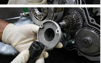
5. Remove the **M6 nut** holding the oil pump drive sprocket. Remove the **sprocket** and **chain**.
