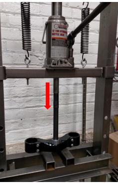
Support the lower fork clamp with suitable parallel bars
