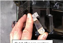
Clutch lifer arm position during cover installation
